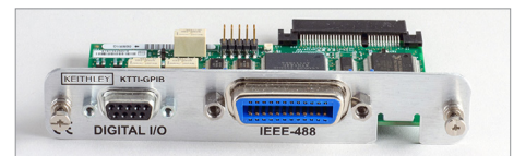
KTTI-GPIB GPIB interface with 6 digital I/O ports.
