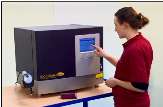
Figure 6 – The operator controls the system via a touch screen
