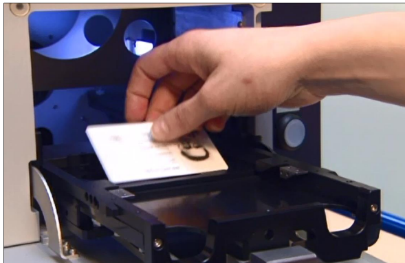
Figure 3 – Adapter for the processing of cards
