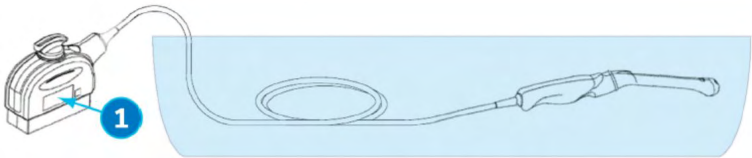
Figure 5-7 Probe Immersion Level for IC5-9-D
