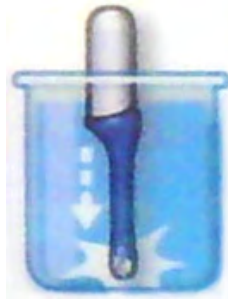
Figure 5-8 Probe suspended in disinfectant basin
