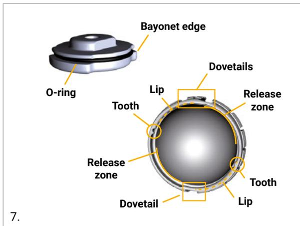
**Step 3:** Position the impacting ring into the shell in the unlocked position (bayonets in the release zones), in order to have:
