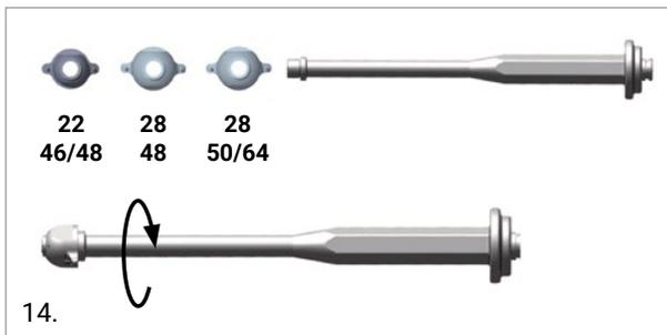
**Step 2:** Assemble the impaction washer with trial fixed liner; introduce and screw the central rod to the last thread in order to stabilize the assembly impactor handle - central rod - trial fixed liner.
