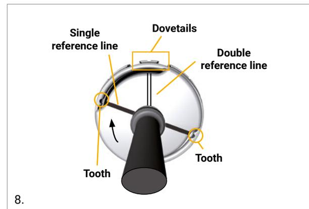
**Step 4:** Correctly couple the two bayonet edges of the impacting ring with the two acetabular shell lips.
