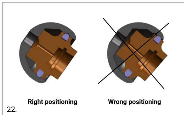
**NOTICE:** The side marked with references of the trial adaptor must stay in the external part of the trial mobile liner.
