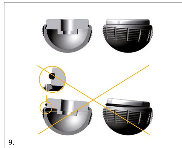
Take care to not damage the inner mirror polished surface of the shell.
