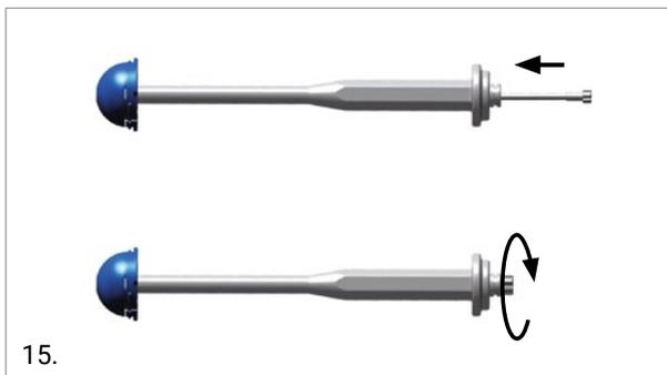
**Step 3:** The assembly is positioned in the acetabular shell by putting two trial liner bayonets in the two release zones and achieving close contact. Lock the assembly into the acetabular shell Versafitcup by turning the impactor handle about 90° clockwise until the two trial liner holes are lined up with the acetabular shell teeth. In the correct position the fixed liner bayonets are completely covered by acetabular shell lips.
