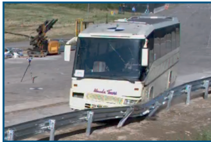
TB 51 Crash-Test Coach 13.000 Kg., at 70 Km/h and 20°
