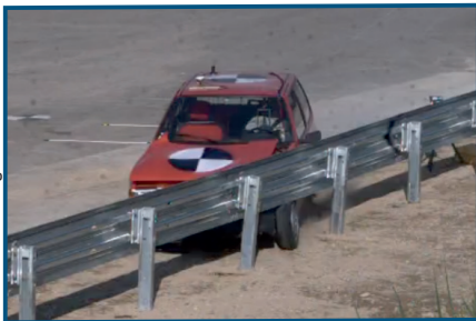
TB 11 Crash-Test Car 900 Kg., at 100 Km/h and 20°
