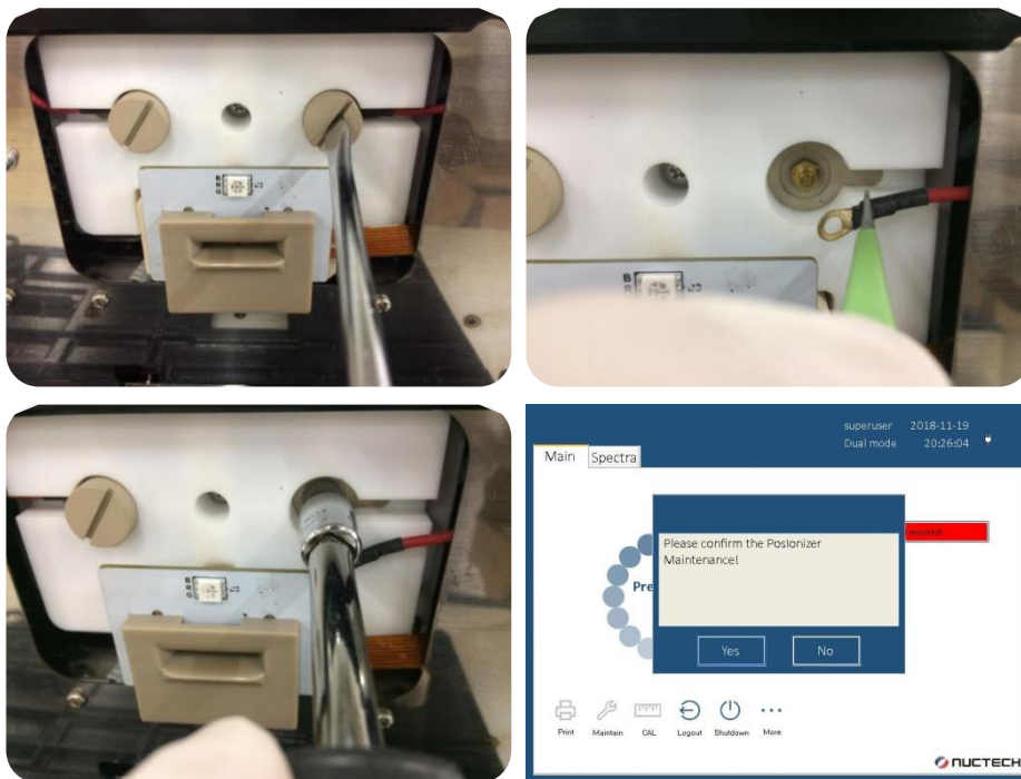
Figure 6.12 Change Ionizer Electrode and confirm afterwards
