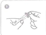
Select the depth of penetration by turning the adjustable tip in either direction so that the arrow on the cap points to the desired depth.
