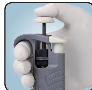
Rotating pipetting pushbutton prevents accidental volume change
