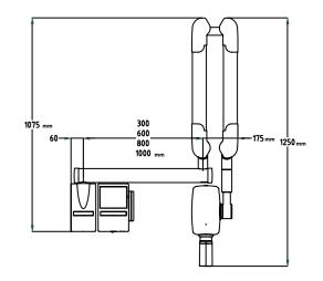
Wall mounted version available in four different extension arm lengths: 30cm, 60cm, 80cm, 100cm
