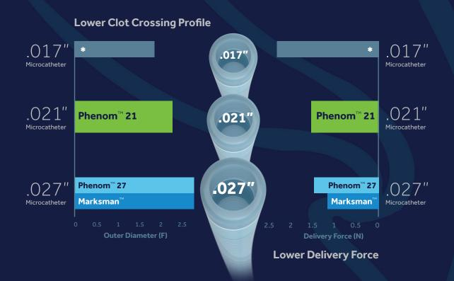
The 3mm Solitaire™ X is designed to be delivered through an 0.017" microcatheter for a lower clot crossing profile or an 0.027" microcatheter for lower delivery force.
