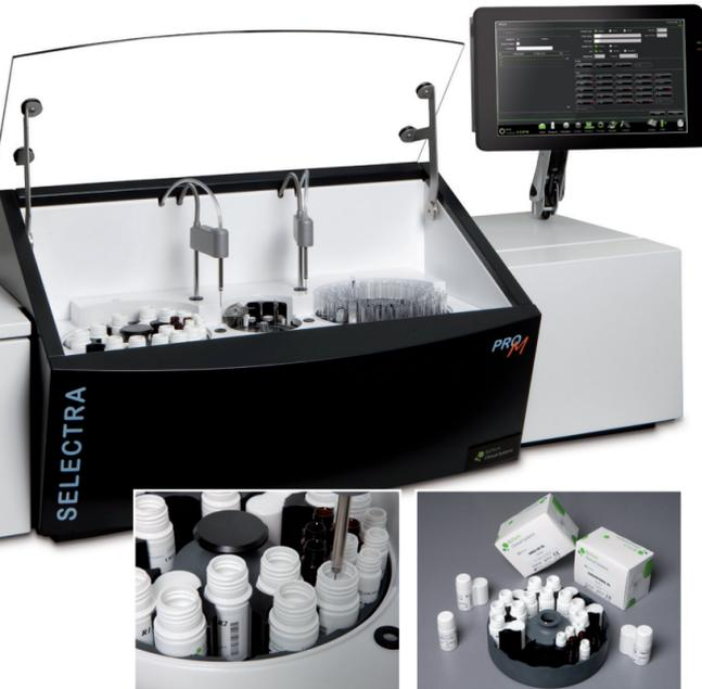
With random access throughput up to 266 tests per hour, the Selectra ProM System is the ideal BenchTop workhorse for primary, STAT or back-up testing needs. This new system offers minimal maintenance and effective use of consumables to truly reduce operational cost.
