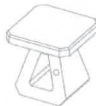
Free standing concrete chair
