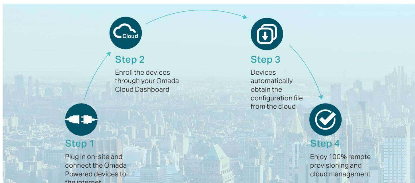
1. Zero-Touch Provisioning is supported when using Omada Cloud-Based Controller
