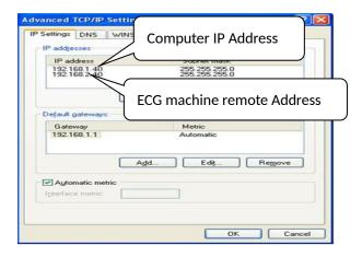
Figure 6-15 Computer IP Setup
