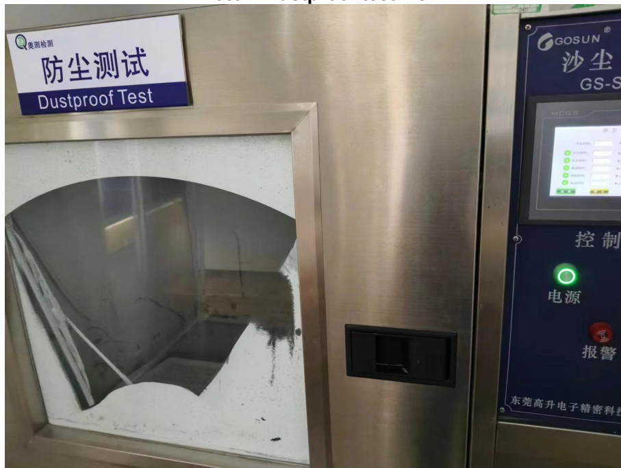
Photo 4 Dustproof test view
