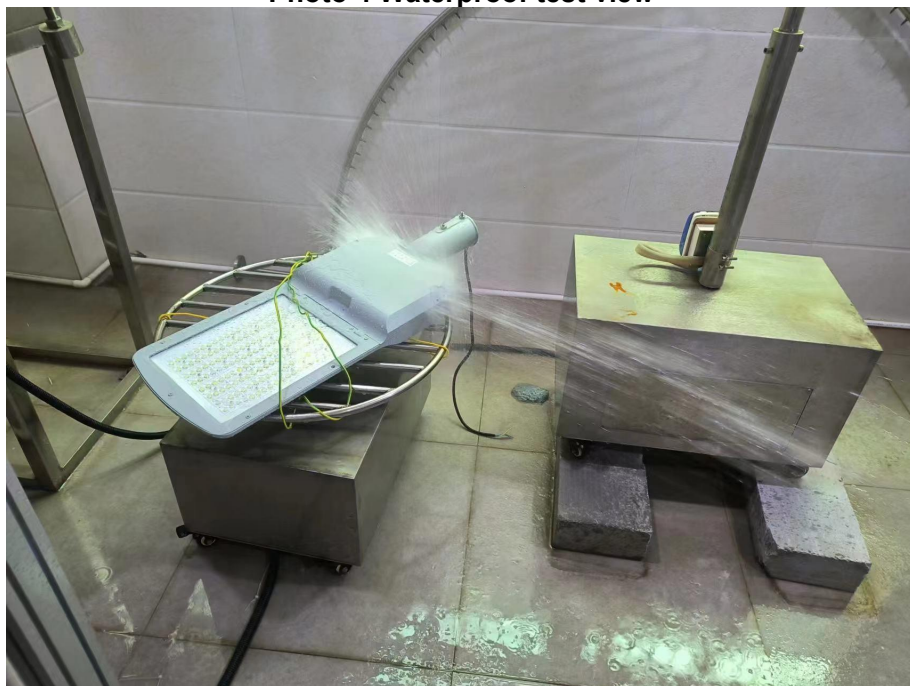
Photo 4 Waterproof test view
