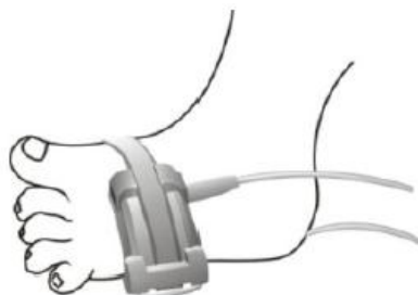
Fig 16-4 Placement of Neonatal SpO 2 Sensor
