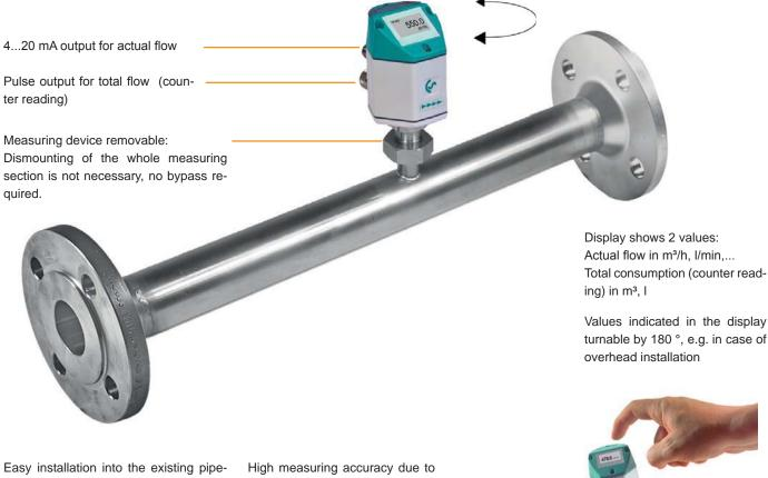
Easy installation into the existing pipeline due to integrated measuring section and weld neck flange (according to EN 1092-1 PN 40) High measuring accuracy due to defined measuring section (inlet and outlet section)
