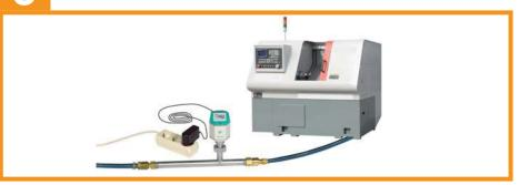
By means of quick couplings the flow meter can be integrated quickly into the feed hose of a machine. During the shutdown of the machine it is possible to determine the leak rate, the actual flow can be obtained when the machine is running. The power supply is effected via the power socket by means of the mains unit. For data recording over a longer period of time we recommend to use the compressed air analyzer DS 400 mobile
