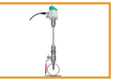
The approved flow sensor VA 400 is available for pipe diameters of 2" to DN 300. Its constructively sophisticated design enables the installation into pipes with nominal diameters up to DN 300 even under pressure. The installation is effected by means of standard 1/2" ball valve.
