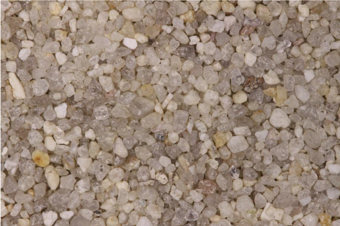
Stabilising Infill - picture
