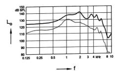
Max. Output sound pressure level  $(L_i = 90 \text{ dB})$
