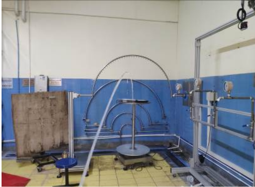
Photo 4 -- During the test of IPX5
