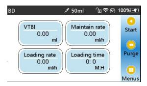
The Loading dose mode means to infusion with the Loading flow rate according to the Loading time, after reaching the Loading time, it works at the Maintain rate till complete the VTBI( Volume to be infused).
