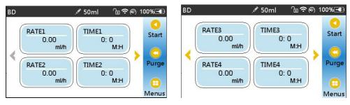
Sequence mode means to perfuse according to the set sequence after setting the rate and time of different sequence groups. At most 5 sequence can be set in this mode.
