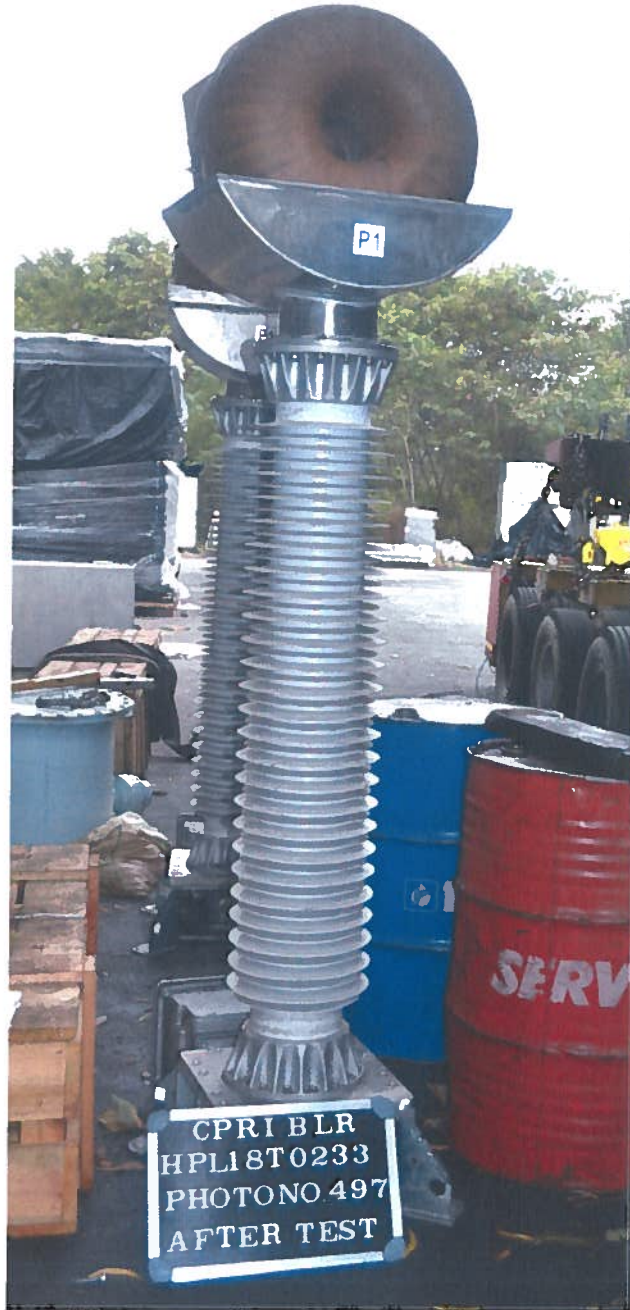
Photograph No. 497: Condition of core, conductor after short circuit test
