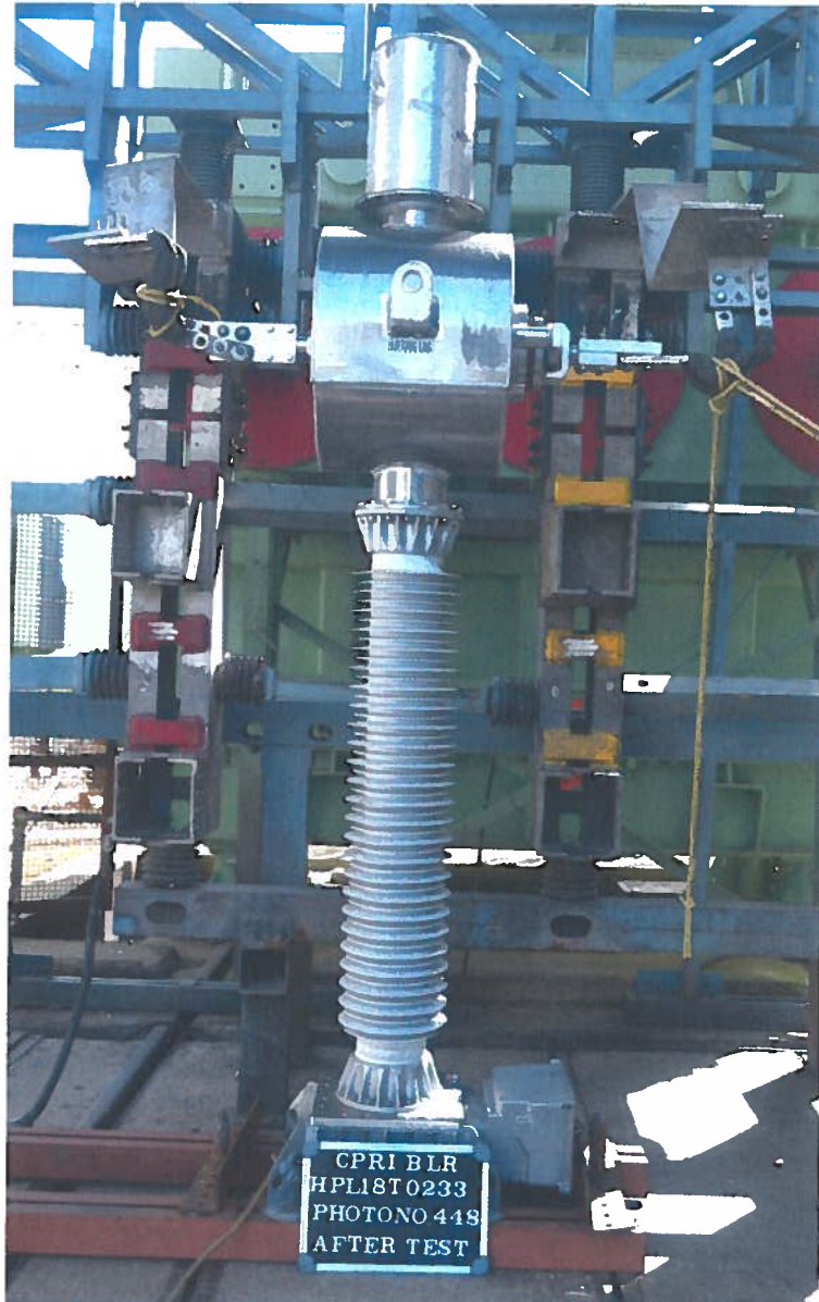
Photograph No. 448: Condition of sample after short circuit test
