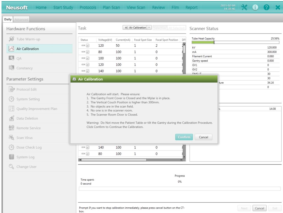
Fig 4-2 Air Calibration
