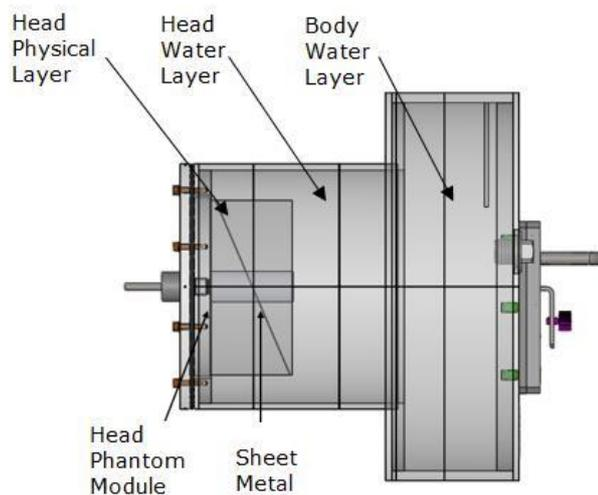
Fig 12-1 QA Phantom Composition
