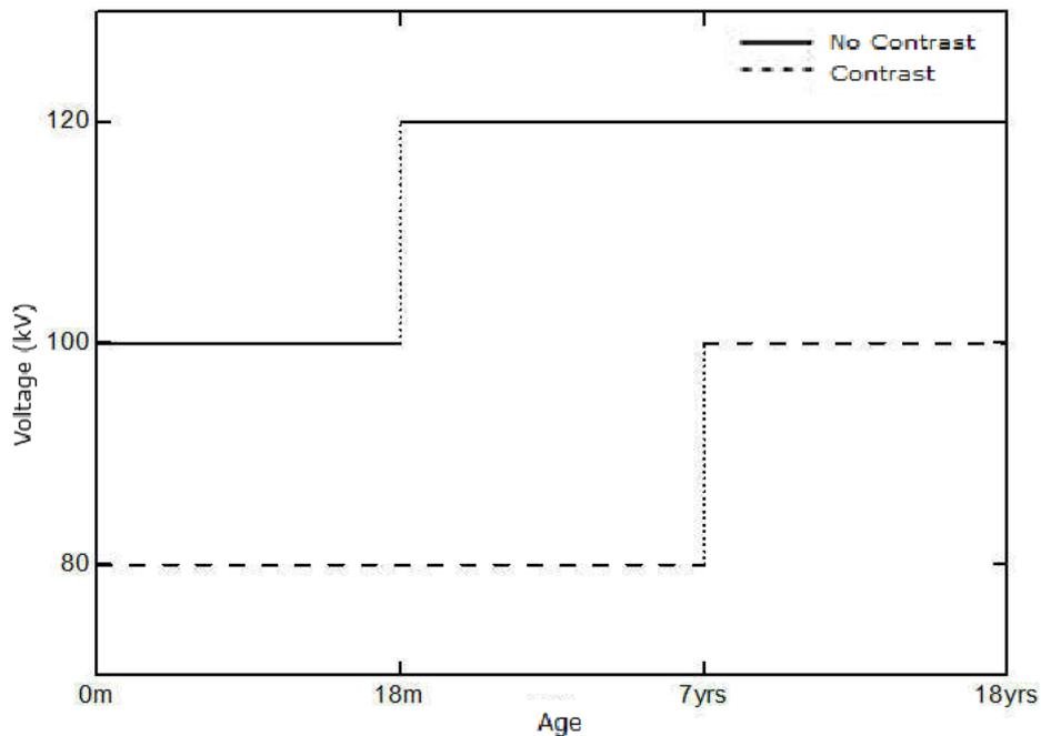
Fig 6-4 kV used in child head protocol
