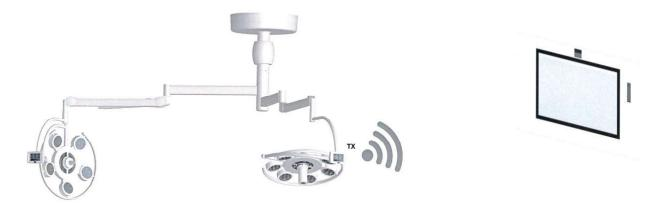
Ensure that a mains socket for the power supplies of both the monitor and the receiver is available nearby.
