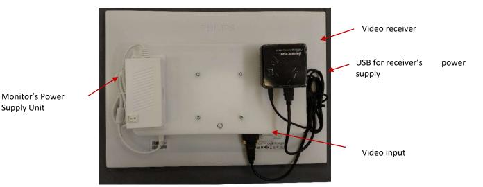
Picture shows the (back) monitor assembly (example, cabling may be different depending on the monitor). Monitor is provided with power supply unit and video receiver.
