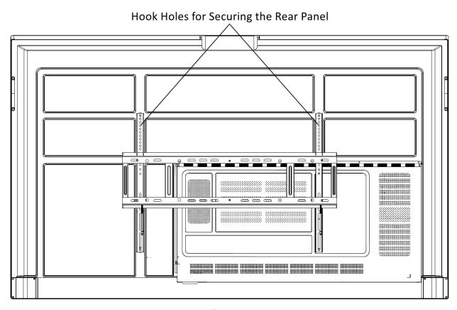
Figure 3-4 Wall Mounting Rear View
