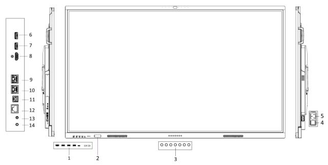
Figure 3-1 Front Panel and Interfaces
