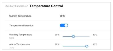
Figure 6-12 Intelligent Temperature Control
