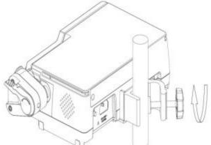
3. Clockwise screw on the clamp knob and ensure that the pump is securely fastened to the pole.
