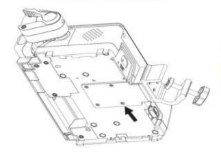
Align the holes of the mounting Bracket with the screw holes on the bottom of the pump and tighten the screws.
