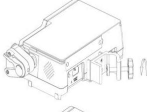
2. Unscrew the clamp knob to fit it to the pole by rotating anticlockwise.
