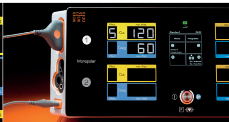
Plug & Cut: The ARC 350 automatically detects that a standard instrument is connected
