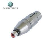
3 pole XLR female - RCA / phono socket Wired according to IEC 268-12: Pin 2: signal; Pin 1 and 3: connected to ground
