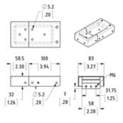
1U Steel Rack Maker, for making 1U Rack Cases. Functions as a Dish, Corners and Braces. Includes a 1U Rack Mount Bracket, Threaded for M6 Rack Screws. Works with L0565 Latch and F0698 Stacking Foot.
