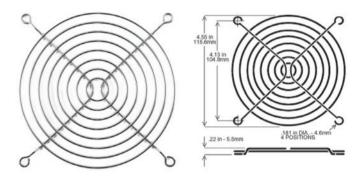
114.3mm / 4.5" Diameter Fan Guard for **P1800** (p.108) and **8700** (p.108)
