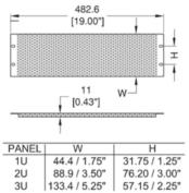
Flanged Perforated Rack Panels. Allow for 62% free air.
