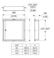
In wall rack cabinet for cavity walls. Available with M6 or 10/32 threaded rack rail. Lockable polycarbonate door Material: Steel & Polycarbonate
