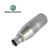
3 pole XLR male - BNC socket Wired according to IEC 268-12: Pin 2: signal; Pin 1 and 3: connected to ground
