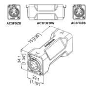
Amphenol D shell XLR in-line adapter 3 pole female to 3 pole female Pre-wired
