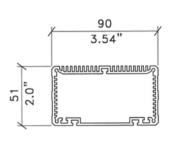
2U All-Purpose Heat Sink Box. Suitable for electronic applications - P.C. Mounts/D.I. Boxes Available in Custom Lengths.
