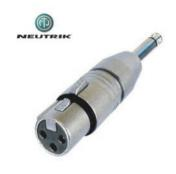
3 pole XLR female - Mono 1/4" plug (tip, sleeve contact) Wired according to IEC 268-12: Pin 2: signal; Pin 1 and 3: connected to ground
