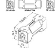
Amphenol D shell SP in-line adapter 4 pole female to 4 pole female Pre-wired
