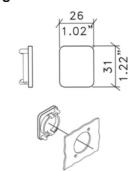
Blanking Plug for XLR/Neutrik D-Series Connector cut-out.
