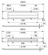
Rack Panel with Cable Access Slot and Brushes. New and improved design with extruded aluminum body.
