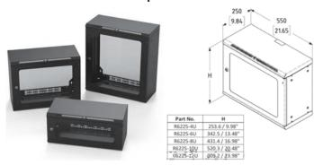
Wall Mount Rack, 250mm / 9.84" Deep, with M6 Threaded Rack Rail Removable outer skin for easy access. Cable Knock-outs in Top and Base.
