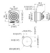
Amphenol RCA Chassis Connector with Red Insulation
