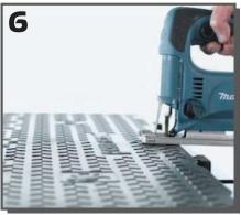
Cross 5 can even be cut into two using a compass saw. This allows you to create even more crossover structures.
