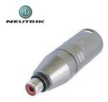
3 pole XLR male - RCA / Phono socket Wired according to IEC 268-12: Pin 2: signal; Pin 1 and 3: connected to ground
