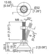
Set of 4 Steel Adjuster Feet with M8 thread for Rack Enclosures. Use with R8230 (p.20) Open Tower Rack System, R2020 (p.15) Modular Rack Tower, R8200 (p.18) Open Rack Tower System, R8400 - R8500 (p.10) Flat Pack Rack System, R6400 (p.21) and R6600 (p.23) Wall Mount Racks.
