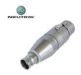
3 pole XLR female - BNC socket Wired according to IEC 268-12: Pin 2: signal; Pin 1 and 3: connected to ground
