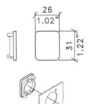
Blanking Plug for XLR/Neutrik D-Series Connector cut-out.
