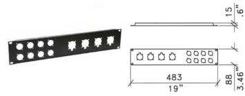
2U Panel punched for 4 x EP Series/Neutrik G-Series Speakon Connectors\* and 8 x Neutrik D-Series Connectors (XLR, Speakon, RJ45, etc.)
