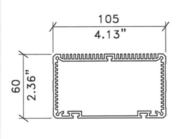
3U All-Purpose Heat Sink Box. Suitable for electronic applications - P.C. Mounts/D.I. Available in Custom Lengths.
