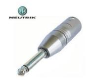
3 pole XLR male - Mono 1/4" plug (tip, sleeve contact) Wired according to IEC 268-12: Pin 2: signal; Pin 1 and 3: connected to ground
