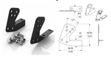
Brackets for mounting 1U Equipment to rear of R1297 Shelf. Can be mounted Horizontally or at 45° Includes 2 Brackets and Fixing Screws.
