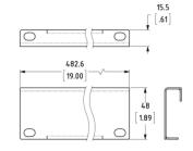
L-Shaped Corner Rack Panels for use with R0863 (p.41) Rack Strip.
