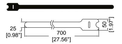
Cable Ties with Hook and Loop Fastening Strips
