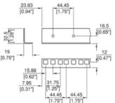
FIXING HOLES 9.5mm/0.38"SQ & Ø5mm/0.20"
