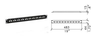
1U Rack Panel punched for Chassis BNC Connectors. Black Powder Coated.
