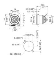
Amphenol RCA Chassis Connectors with Red Insulation
