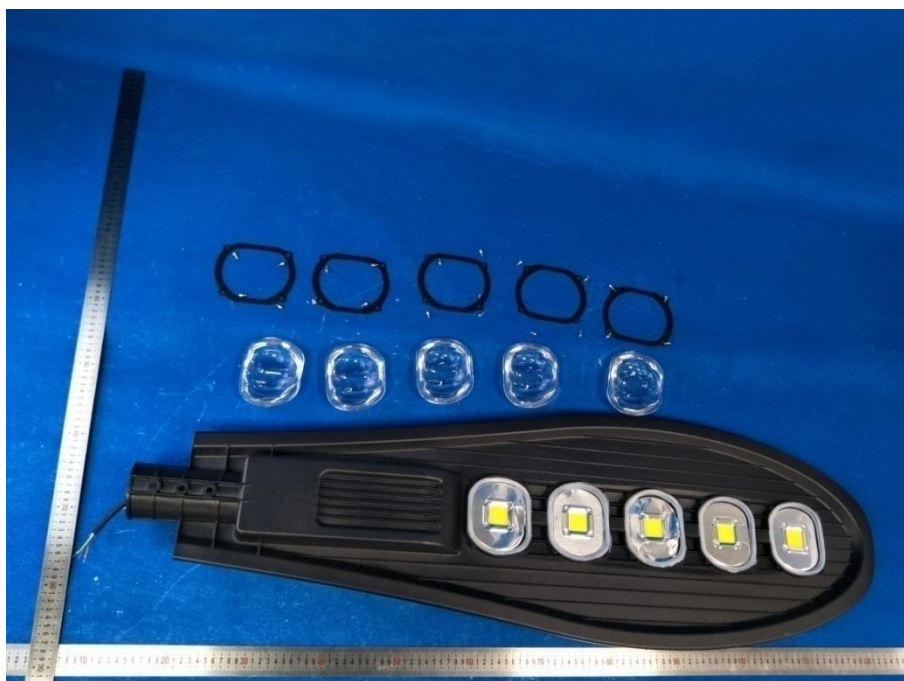
Uncover internal view for CET-124COB-250W
