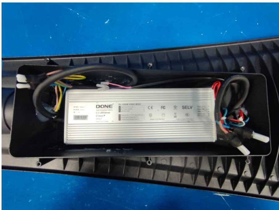
Uncover internal view for CET-124COB-250W
