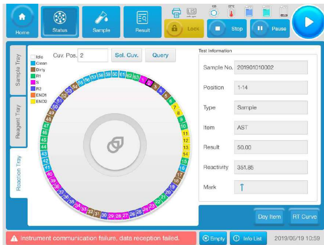
Figure 4-7 Status of Reaction Tray
