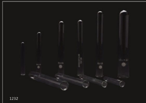
1232 Glass Test Tube With Rim Neutral/Borosilicate 3.3 With / Without Print
