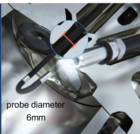
It can insert and inspect as long as there are holes or gaps
