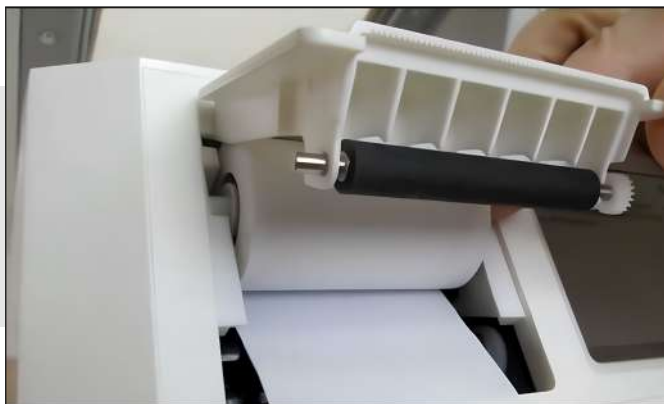
Fig.46. Replacing the paper roll for the built-in printer
