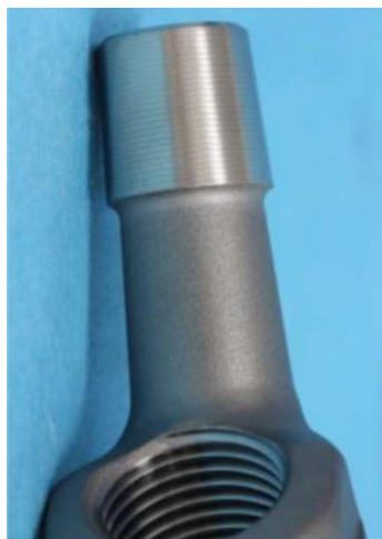
FIGURE 7. 12/14 MORSE-TYPE TAPER TRUNNION AND THREADED HOLE FOR THE SAFETY SCREW
