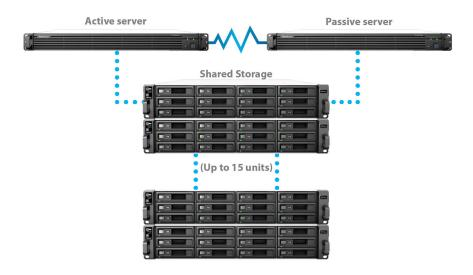
The connected RXD1215sas acts as the shared storage pool of the two servers, so no data replication is required, saving more energy and rack spaces. The storage capacity is expandable by adding more RXD1215sas (up to 15 sets) to the HA cluster, providing the scalability up to 180 HDDs and a maximum raw capacity beyond 1 petabyte.
