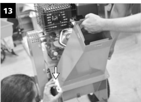
**EN** Attach the removal channel (4x M8). The removal channel is not side-dependent, so it does not matter how it is attached. Attach the chimney of the removal channel and fasten with buckles/screws (depending on the type).
