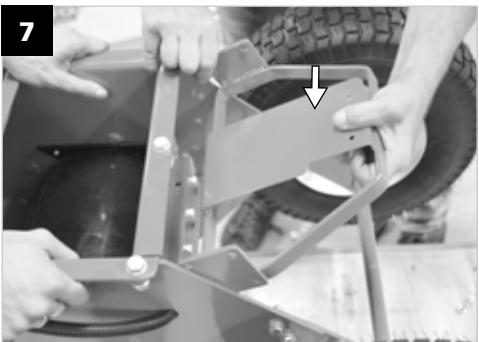
**EN** Install the battery base (4x M8). Tighten the wheel axle and the battery base firmly.
