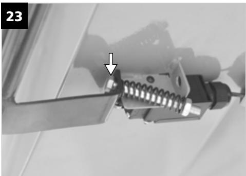
**EN** Pass the screw through the ring hole, put the spring on it and install the locknut so that the spring is not loose and is slightly compressed by the nut. Fit the screw back into the filling channel and firmly tighten.
