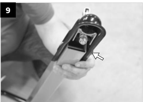
**EN** Attach the drawbar to the shaft and tighten it firmly. Take down the shaft with the front girder and tighten by butterfly screw.
