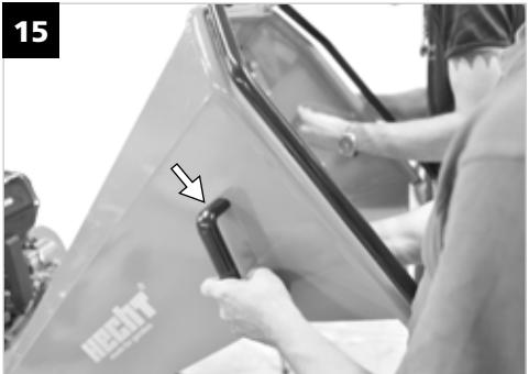
**EN** Attach the handles on the filling channel (handles, screws and washers can be found in the tool case). Fasten the filling channel to the machine body (5x M8). After tightening the filling channel, connect the stop button connector at the bottom.
