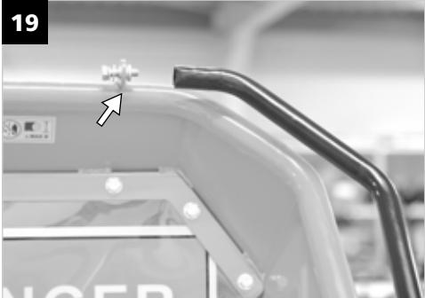
**EN** Place the fitted washers into the holes at the top of the filling channel as shown in Figure (FIG. 20) by fitting towards the ring. Install the ring.
