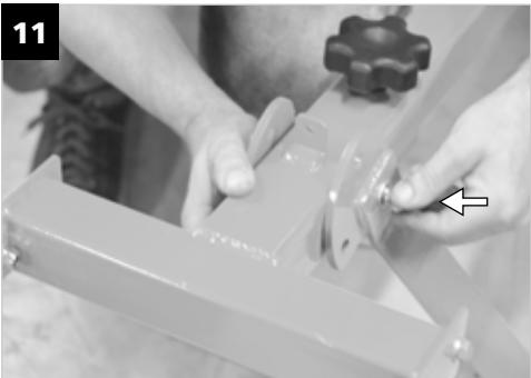
**EN** Install the front support on the front girder with the shaft (4x M8). Lift the machine on the removal channel side and attach the front girder with the shaft. Tighten it all.
