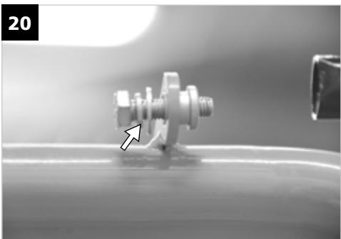
**EN** Remove the long spring screw at the top of the filling channel (M8 x 80). Remove the locknut and lower the spring.
