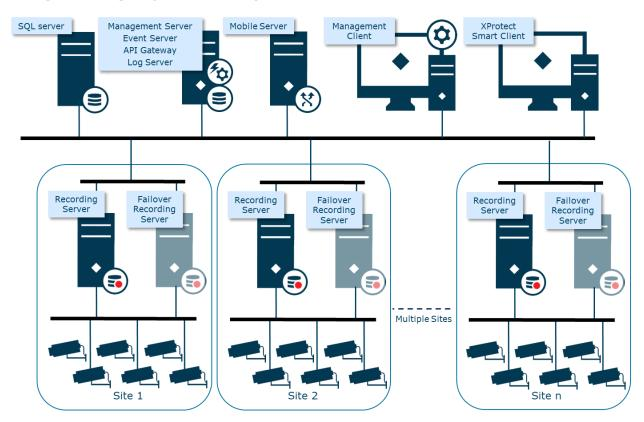
This design is essentially the same as design 3. The only difference is that the cameras and recording servers are located on physically remote sites, and not on the main site where the management server and the VMS users are located
