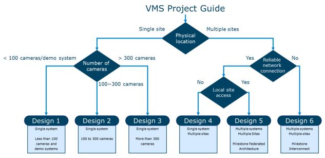
**Note:** The 'Number of cameras' decicion limits are based on cameras set to: H.264/H.265, 1080p, 25/30 FPS and a bitrate of 3-5 Mbit/s.
