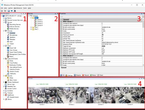
The Management Client has a "Site Navigation" area (1), where nodes for various parts or functions of the system can be selected, for instance 'Cameras' as shown on the screenshot above.
