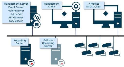
To provide live and recording capabilities in scenarios where the recording server has failed or is stopped for maintenance, a failover recording server can be added.
