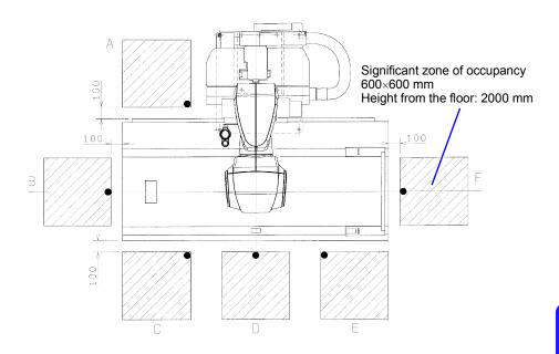
The following graph shows the stray radiation doses measured at the points marked with  $(\bullet)$  in the figure above.
