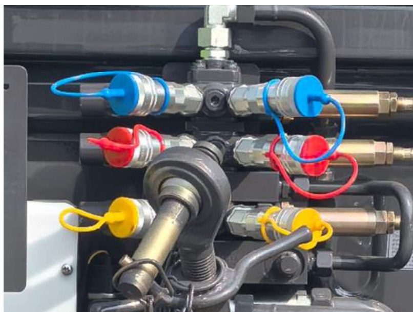
Identification of hydraulic couplings
