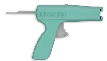
The dispenser gun consists of a pistol type, ergonomic handle with an integrated barrel and trigger. Each depression and hold of the trigger delivers a 0.3 cc in 5 seconds continuously.
