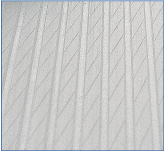
Magnification of a skin graft carrier plate with its fine grooves.
