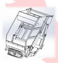
Tailgate connected to body with top hinges. The tailgate structure is consist of 1 sledge, 1 shovel, hopper and their cylinders. When garbage is put inside the hopper, with the help of the sledge and shovel this garbage goes into body and compressed with pushout plate. Sledge moves linearly and shovel moves radially to sweep the garbage inside the body, the sledge runs on sliding rails with roller or shoes.
