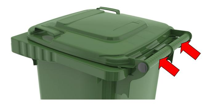
■ Two extra grip areas of equal size are attached to the body in the form of a continuous, ergonomically well-shaped grip tube in wave geometry via a triple body connection. The grip tube with a diameter of 27 - 28mm, lies comfortably in the hands and thus even full bins can be manoeuvred safely.
