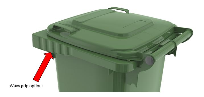
■ The bins are predominantly positioned with the handle tube facing the wall, so that it is then not possible to move the bin the first metre over the handle tube. In order to make it easier for the user to pull the bin out of this position, wave-shaped grip options on the upper, front side edge of the bin were taken into account in its development.
