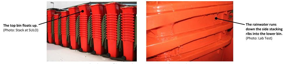
Here are example photos of bins without an optimised water drainage system
