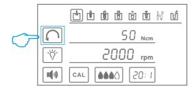
► Touch the arrow location icon, the motor can switch between forward and reverse:
