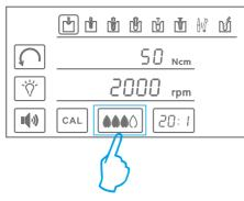
► Touch the coolant display until the supply rate is set as desired;
