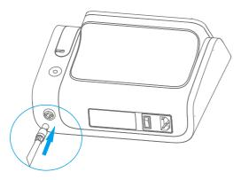
▶ Insert the foot controller plug into the socket on the back of the unit. Make sure that the marker arrows on the plug and the socket are aligned towards each other.
