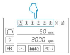
▶ Press and hold the program icon that need to be reset until the Icon flashes and buzzer beep twice to indicate the reset has been completed.
