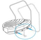
▶ Slide the handle into the designated recesses, and then tighten the nuts by hand.
