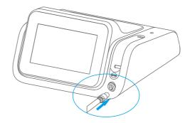
▶ Insert the surgical motor plug into the socket on the front of the unit. Make sure that the marker arrows on the plug and the socket are aligned towards each other.
