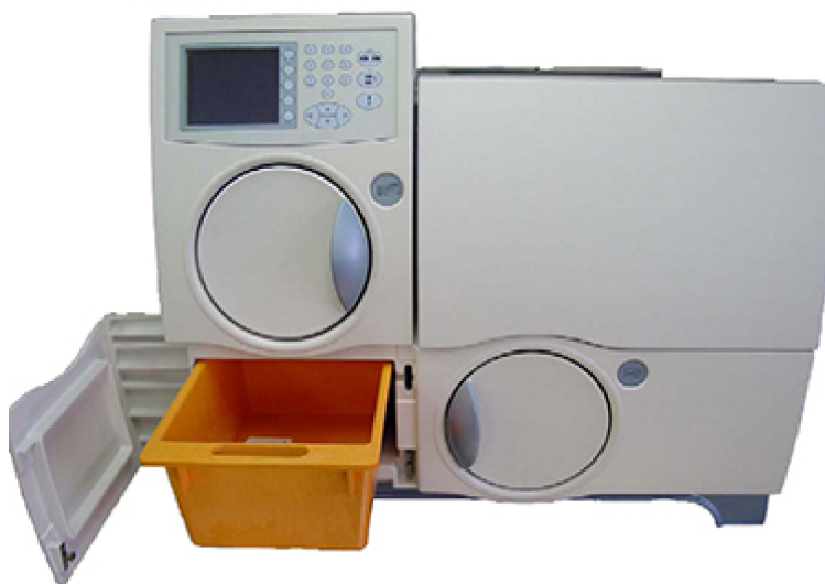
Figure 24: Waste Collection Station
