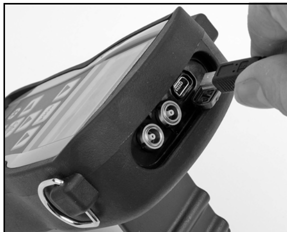
Figure 21: Location of Mini USB COM Port
