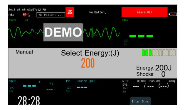
In defibrillation message area at the middle of manual defibrillation interface, such information about manual defibrillation as defibrillation mode, synchronized status, energy level, impedance indicator, defibrillation prompt message, shock times and so on will be displayed.
