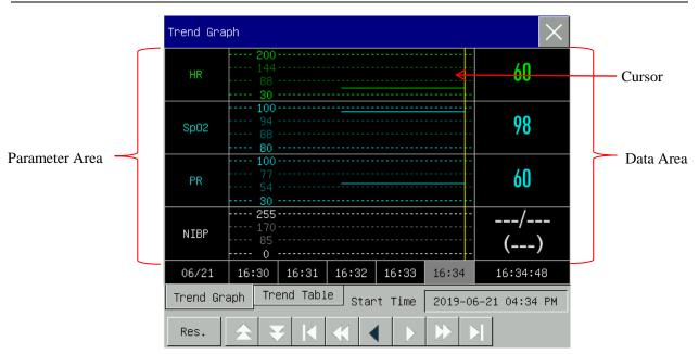
Aperiodic measurements can be viewed from the trend table. This table shows measurement data and measurement time. During a maximum period of 160h, the trend table data can be viewed.
