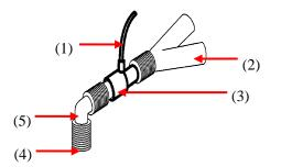
(1) Sampling line (2) Y-shaped tube (3) Airway adapter (4) Breathing tube port (5) Elbow tube
