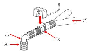
(1) Elbow tube (2) Y-shaped tube (3) Airway adapter (4) Breathing tube port
