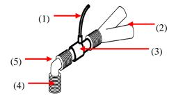
(1) Sampling line (2) Y-shaped tube (3) Airway adapter (4) Breathing tube port (5) Elbow tube
