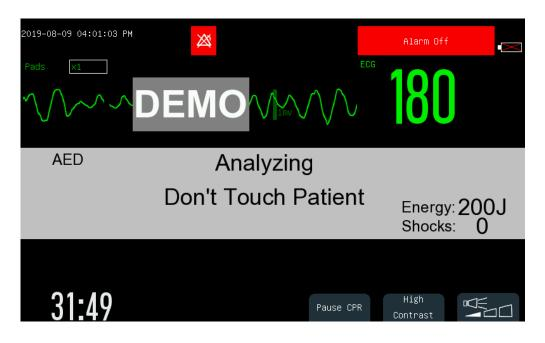
In AED mode, the Defibrillator Monitor will only display one ECG waveform detected by pads and HR value calculated from this displayed waveform. The AED message area at the middle of AED interface will display AED prompt message, contact impedance indicator (settable), shock times and so on.
