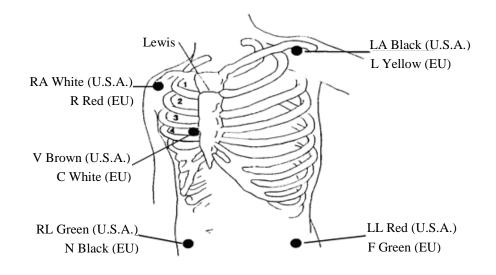
For 5-lead configuration, place the chest (V) lead electrode at one of the following positions:
