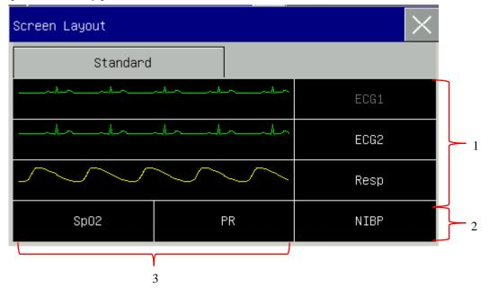
Area 1:Waveform area: You can choose to display the parameters and their waveforms (if one exists). The first row of this area always shows the first ECG waveform and parameter. Waveforms are displayed on the left and parameters on the right. The waveform and its corresponding parameter are shown on the same line.
