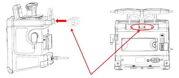
Use four M5 screws to fix the bracket on the ambulance through the hole in the red circle shown in the figure below.
