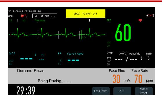
In pacer mode, the monitor can display one ECG waveform and other physiological parameters monitored. In the pacing message area, such information related to pacing as pacing mode shortcut key, pacing message, pacing alarm, pacing current and pacing rate will be displayed.
