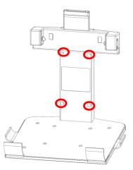
Put the monitor on the bracket, and then tilt it to the wall, and fix the monitor to the bracket through the hole shown by the red arrow below.
