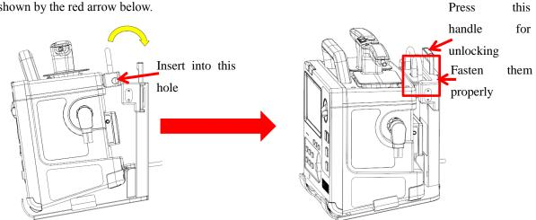
Use four M4 screws to fix the bracket with the host through the hole in the red circle shown in the figure below from the bottom of the bracket.
