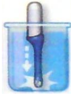
Figure 5-8 Probe suspended in disinfectant basin
