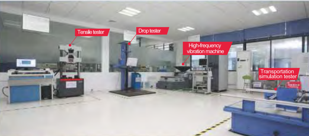
Mechanical Environmental Laboratory Simulate various extremely mechanical environments to ensure the quality of products.
