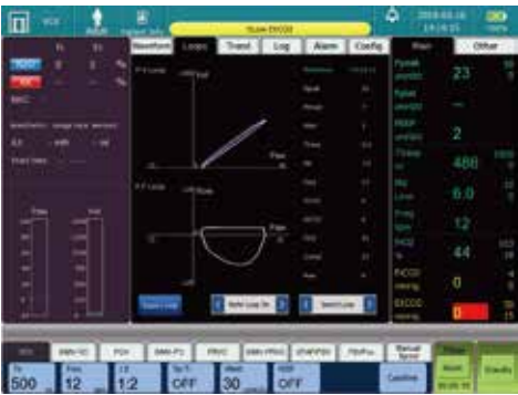
Real time measuring for airway pressures, flow, volumes, compliance and resistance of breath offer a intuitive tool to detect leaking, airway obstruction and optimal ventilated parameters adjustment
